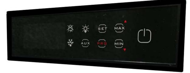
*Top Row left to right:* Alarm Mute, Light on/off, Set Key, Maximum Temperature, Standby Power *Bottom Row left to right:* Defrost, Aux Key, Programming Key, Minimum Temperature, Standby Power **Displayed Symbols:**
